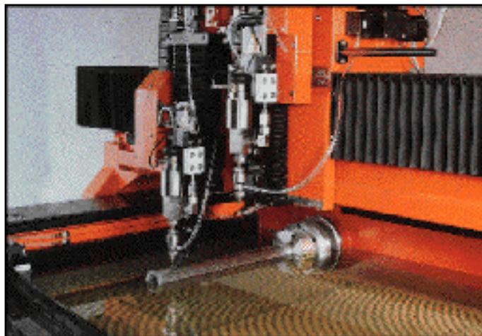
Individual cutting heads on the Bystronic waterjet cutting system, each equipped with automatic height sensing systems and an optimum regulation of the abrasives, result in high cutting quality.
