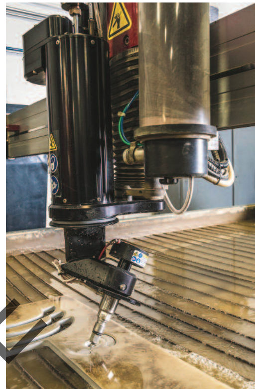
A multiaxis cutting head allows RPM Design to cut angles ranging from 0 to 60 deg. as well as create beveled edges, angled sides and countersinks.
