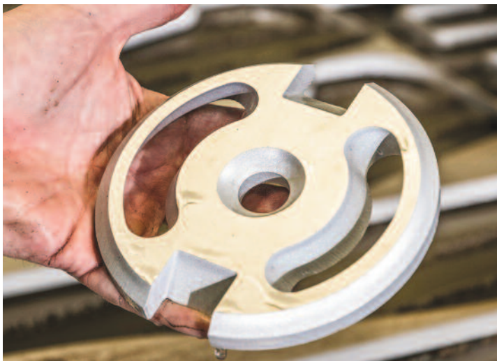
Shown here, one of the complex parts RPM Design produces on its waterjet-cutting machine.
