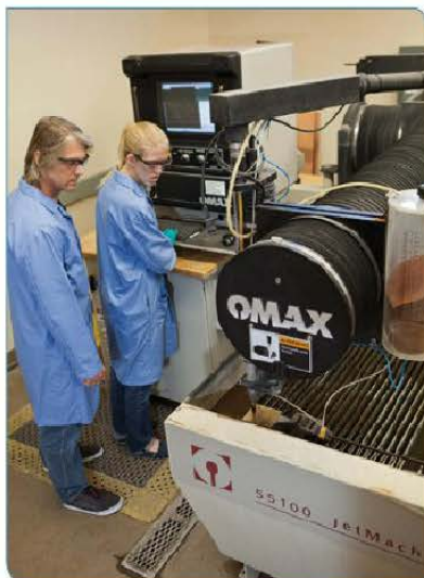
Fig. 2: The High-Performance Materials Institute relies on an OMAX® 55100 JetMachining® Center to quickly and accurately cut a wide variety of components, including carbon fiber composites.
