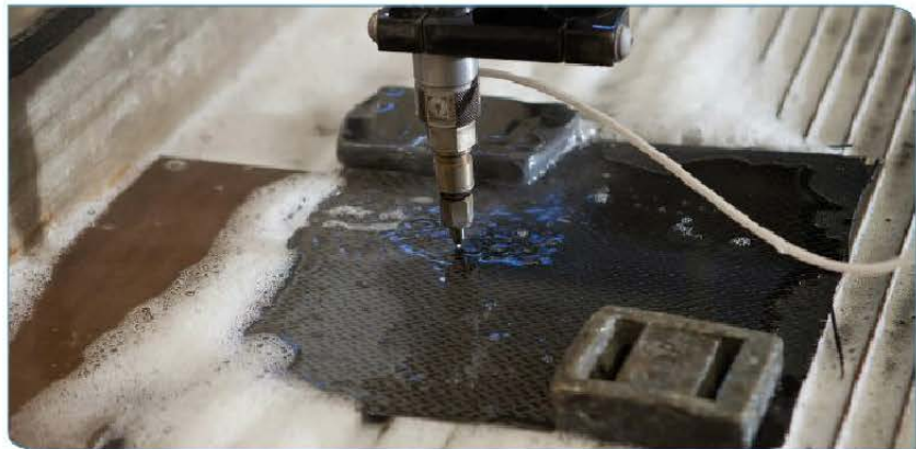
Fig. 3: Composite materials generate a lot of dust when dry cut on a CNC machine, which can be harmful if breathed in. Therefore, the High-Performance Materials Institute relies on the OMAX® 55100 JetMachining® Center to create a cleaner, safer working environment for cutting strong composite materials.
