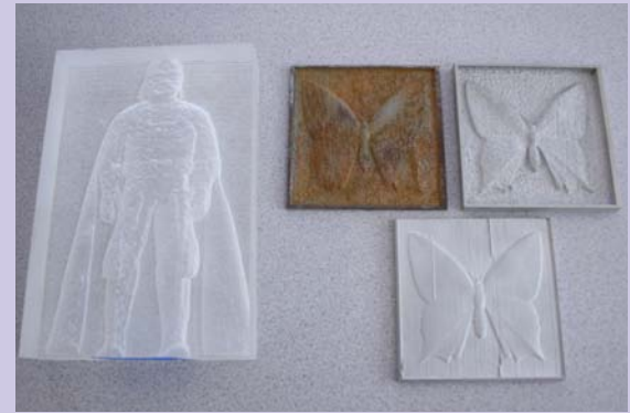
Technicians at Showman Fabricators use the waterjet to emboss artistic elements onto glass, acrylics, and metals.
