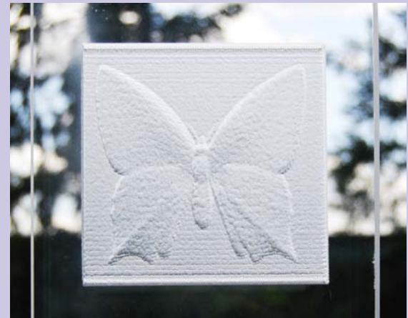
An abrasive waterjet embossed these butterflies onto acrylic. (Photo courtesy of OMAX Corp.)
