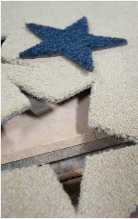
FIGURE 4 Showman's waterjet cut these carpet sections for the White House's new press briefing room.
