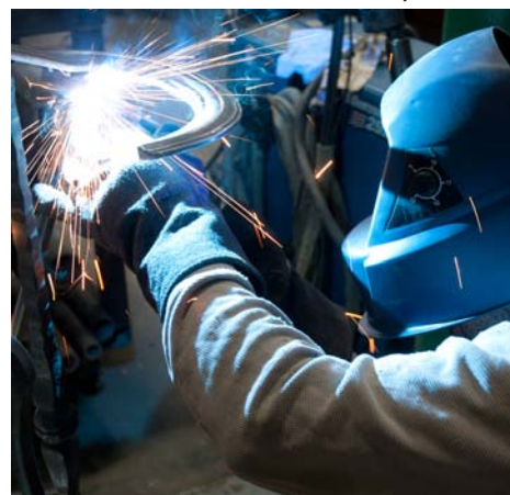
FIGURE 2 A worker in Showman's metal shop welds a metal support onto a set piece.
