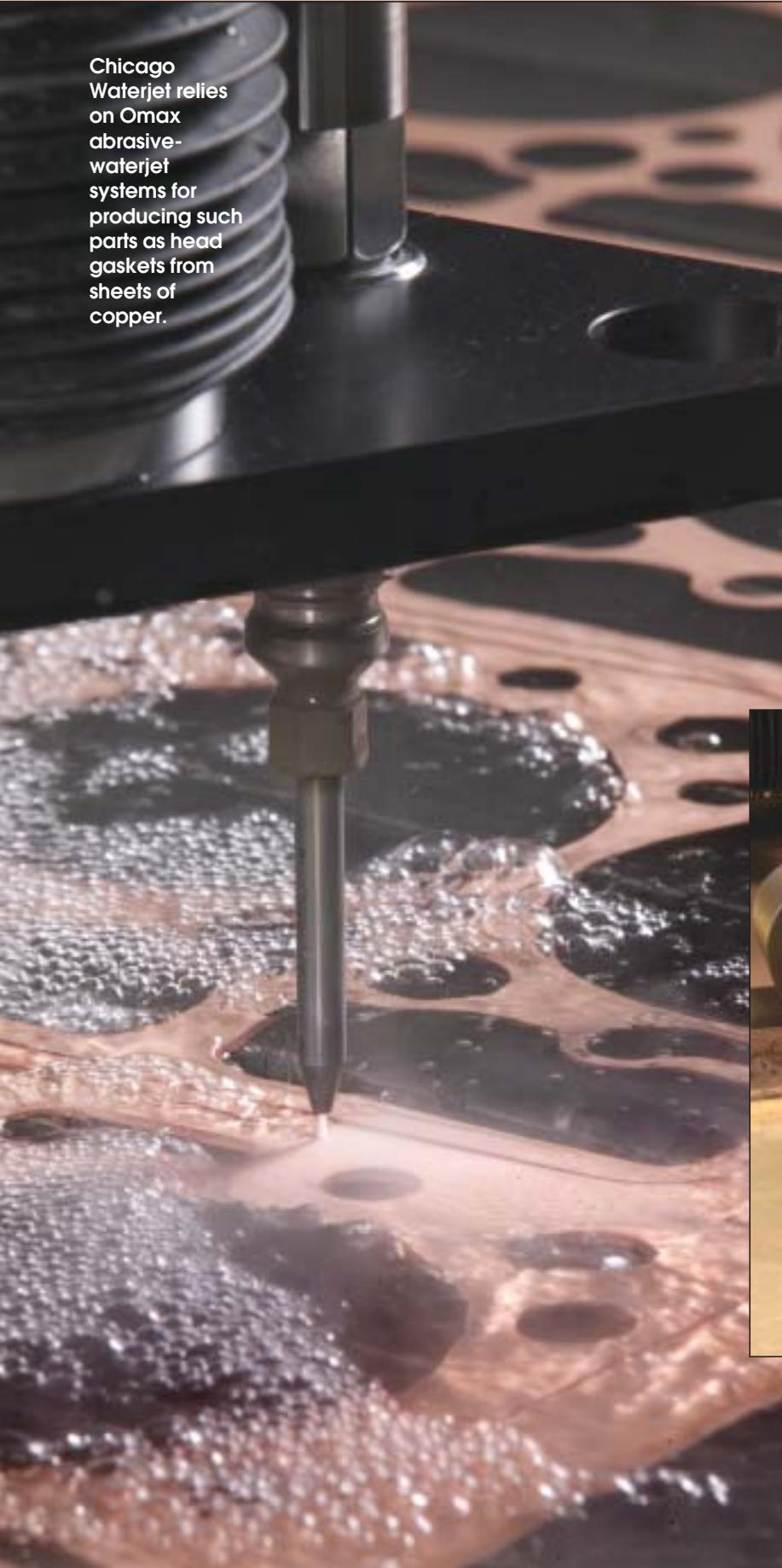
Chicago Waterjet relies on Omax abrasive-waterjet systems for producing such parts as head gaskets from sheets of copper.
