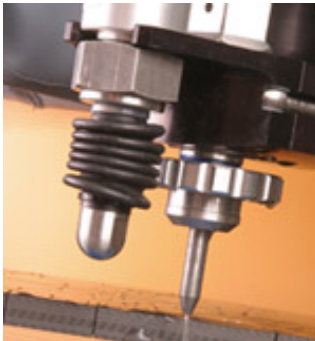
Detail of Flow system cutting layered material.
