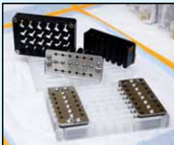
Abrasive waterjet cutting played a key role in producing parts, such as these channel plate assembly components for holding DNA samples, used by the Barracuda robot at the Genome Science Center.
