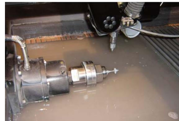
**FIGURE 4** A rotary-axis accessory enables the waterjet to cut bar and tube shapes. Here the waterjet cuts a bar into the shape of the Seattle Space Needle. Photo courtesy of OMAX Corp.
