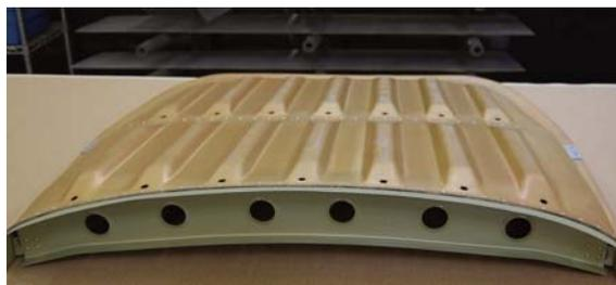
**FIGURE 2** This stretch-formed skin was trimmed on a waterjet system, with the cutting head moving in Z. Photo courtesy of OMAX Corp.
