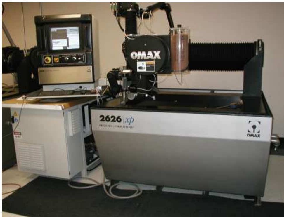
Figure 1 A typical layout of an abrasive waterjet machine
