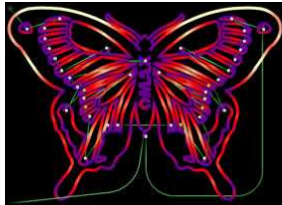
Figure 9 b) Complex velocity profile generated by a cutting model. Speeds are indicated by color ranging from blue (slow) to white (fast).
