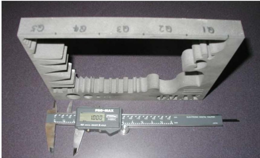
**Figure 19.** An “all-feature” part cut with a tilting head
