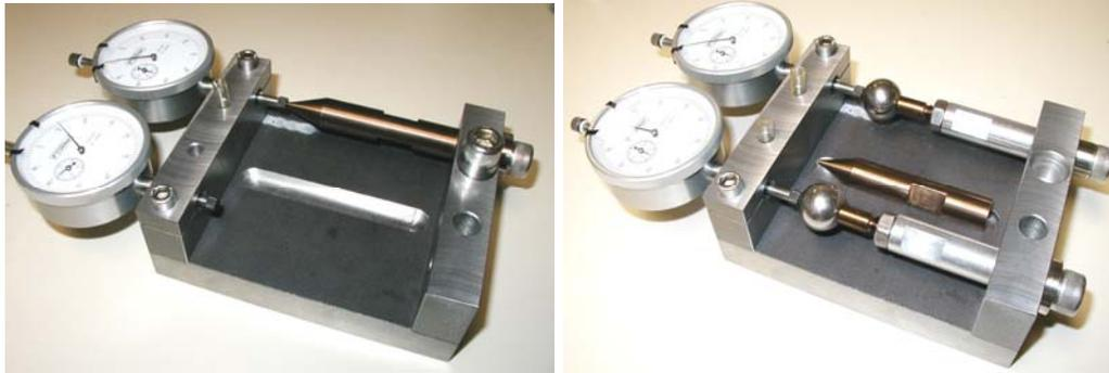
**Figure 16.** Linkage arm calibration tool
