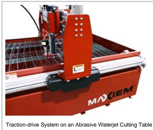
Traction-drive System on an Abrasive Waterjet Cutting Table
