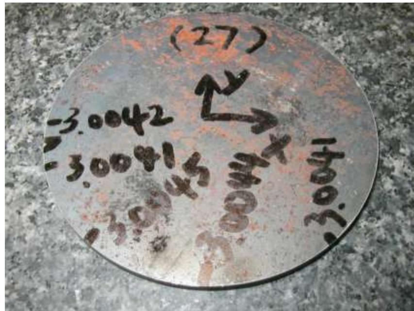
**Figure 7.** Disc cut on material with stress relief.
