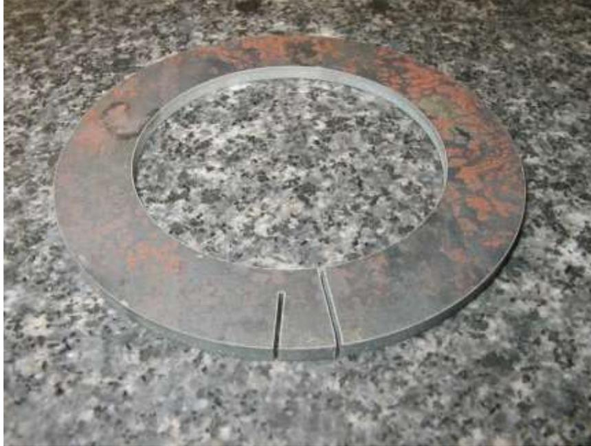
**Figure 9.** Split ring cut on stress relieved material.
