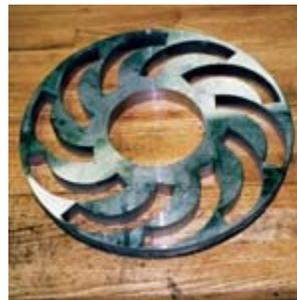
Using an abrasive waterjet machine, blanks for a three-section retainer ring (top)
