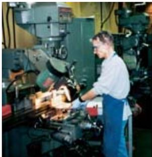
Milling teeth for the tiny jaws of feeder-gripper parts is a precision operation that requires the experience of machinist Ingrid Redding.
