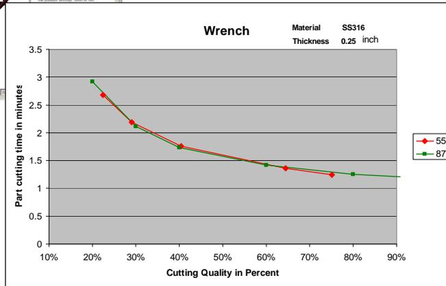
Fig1: A simple part and virtually no difference in cutting time
