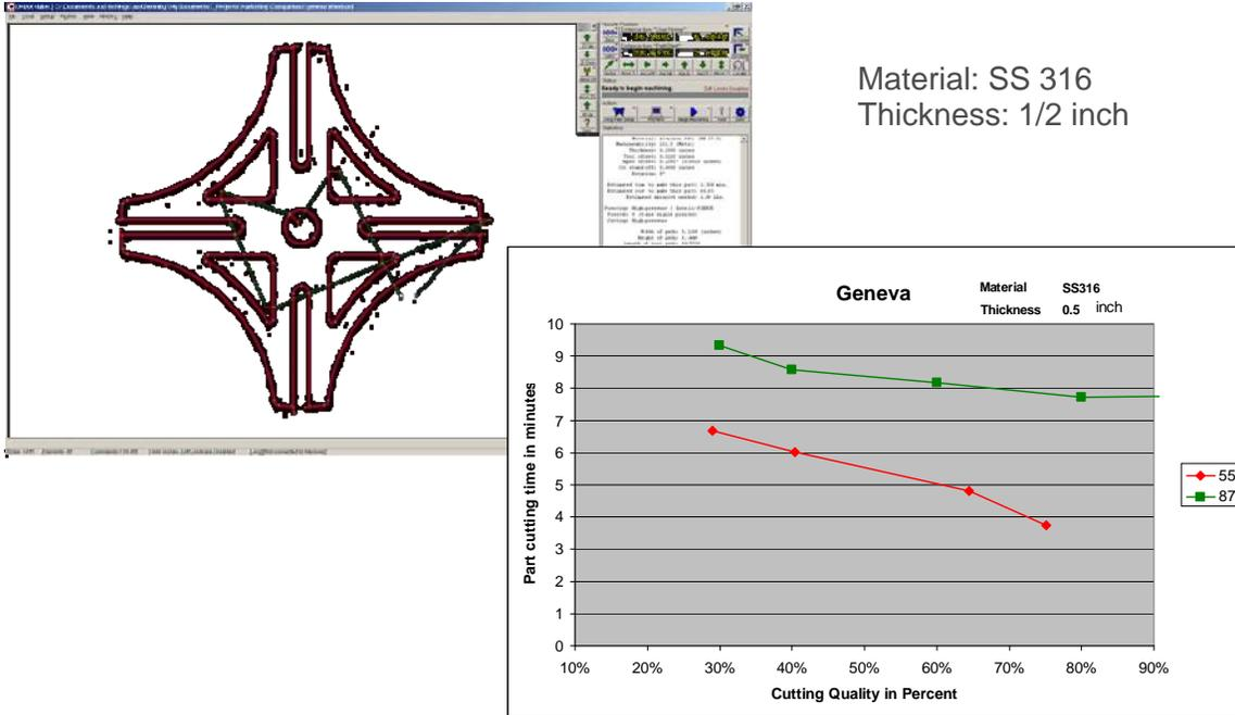
Fig.2—A more complex part shows the clear time benefit of advanced software control
