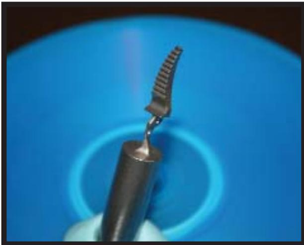
**North-South Machinery produced this medical component by using abrasive waterjet to cut the profile and wire EDM for higher tolerance features and finishing operations.**
