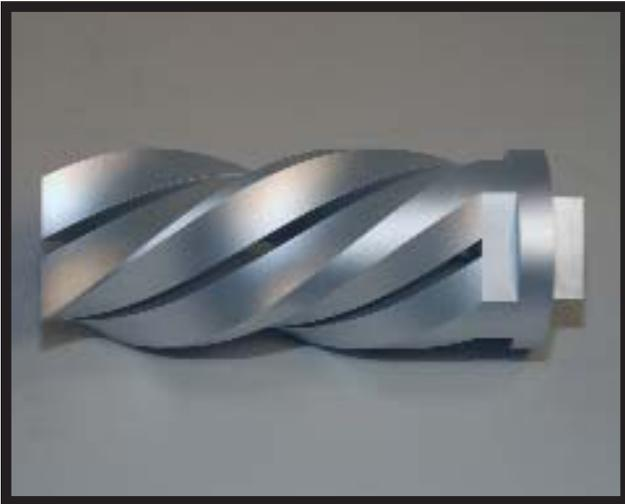
**Though waterjet can only machine in two dimensions, GF AgieCharmilles' Turn while Burn technology enables wire EDM machines to produce complex 3-D shapes.**
