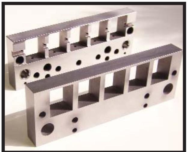
**Using a combined wire EDM and abrasive waterjet machining process reduced the production of this die frame component from 6 to 2 hours.**
