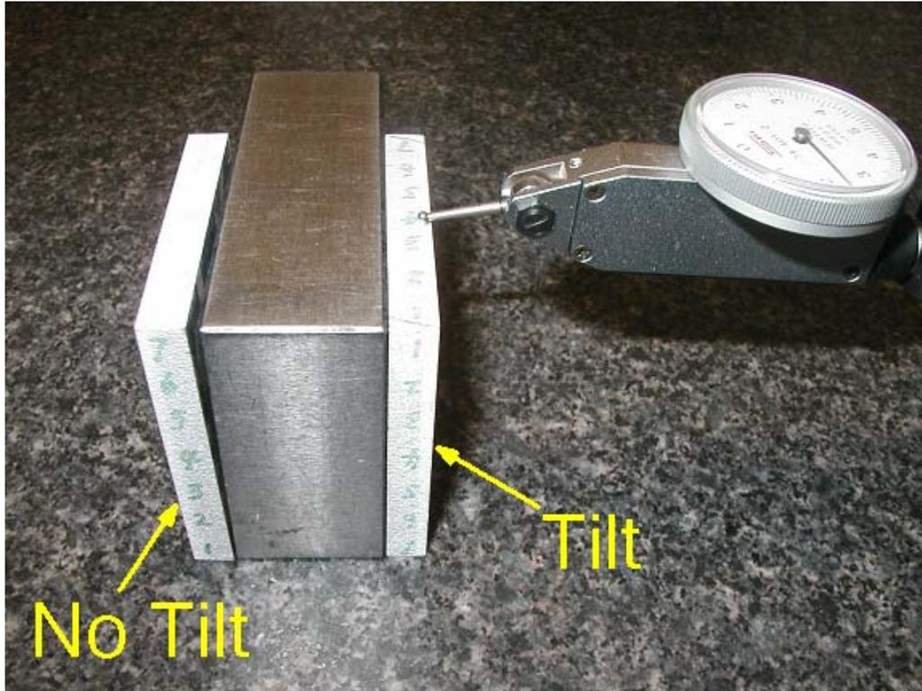
**Figure 11.** Samples cut with and without the tool tip tilting mechanism
