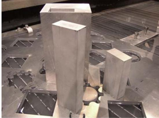
**Figure 3.** A 20 cm (eight inch) thick aluminum rectangle machined using corner passing to improve the quality of the outside corner, while simultaneously speeding up part cutting significantly
