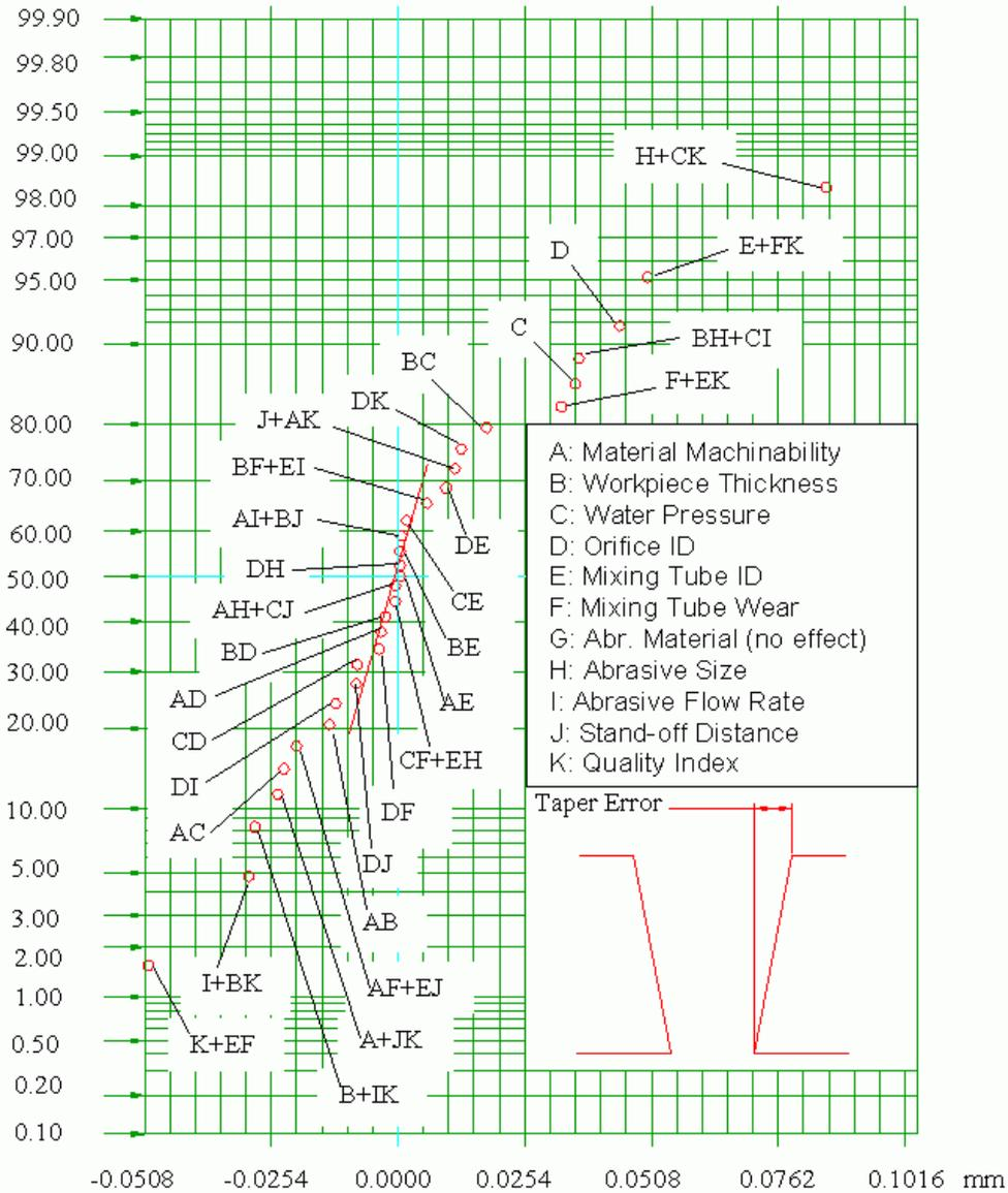
**Figure 9.** Effects of process parameters on taper error
