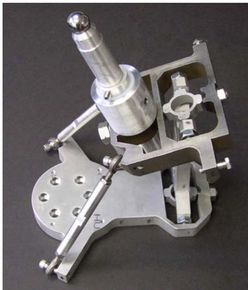
**Figure 7.** Early prototype of tool tip tilting mechanism
