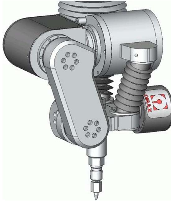
**Figure 8.** Solid model of final design for tool tip tilting mechanism
