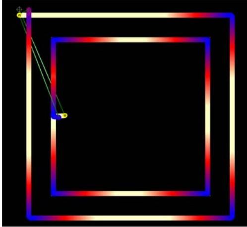
**Figure 1.** With no optimizations other than basic corner compensation, the part takes 17.1 minutes to machine.
