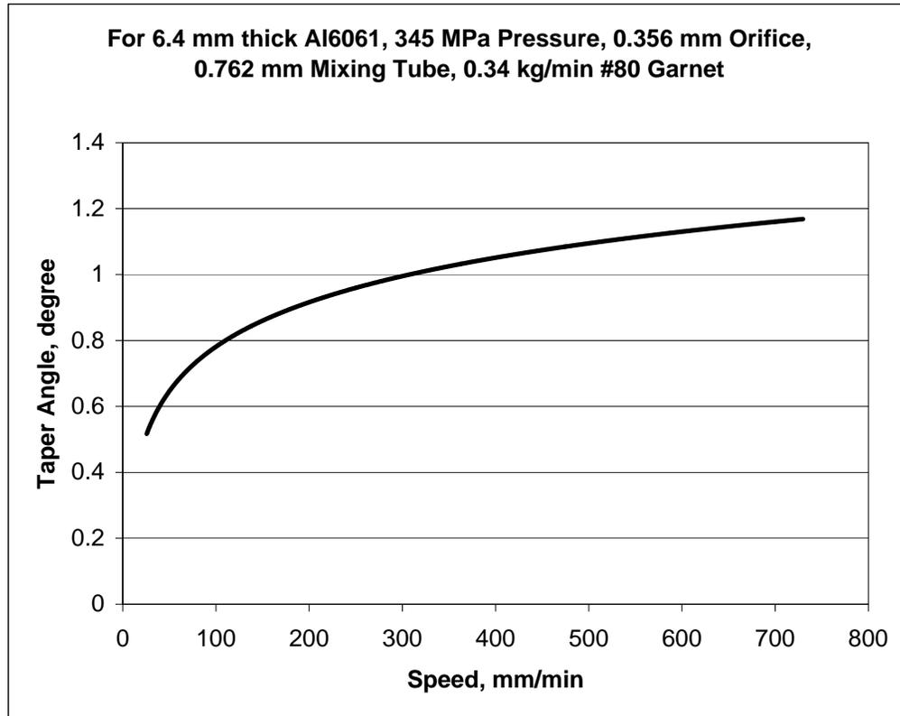
**Figure 5.** Taper angle as a function of speed
