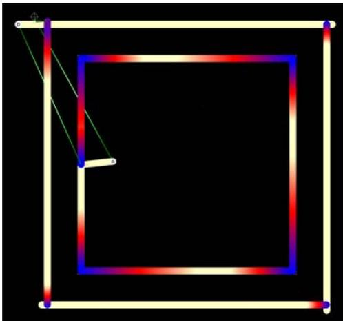
**Figure 2.** With the addition of optimized dynamic piercing, corner strategy, and corner passing, machining the part speeds up to 13.7 minutes.
