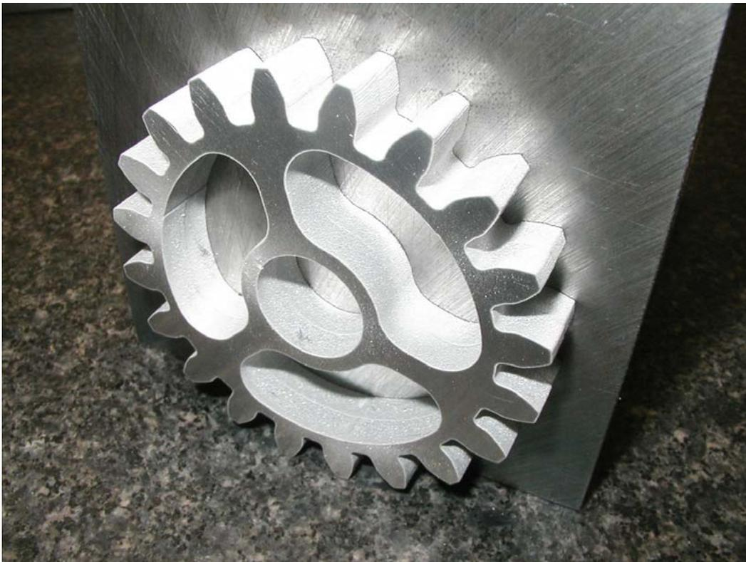
**Figure 12.** Gears cut with tool tip tilting mechanism
