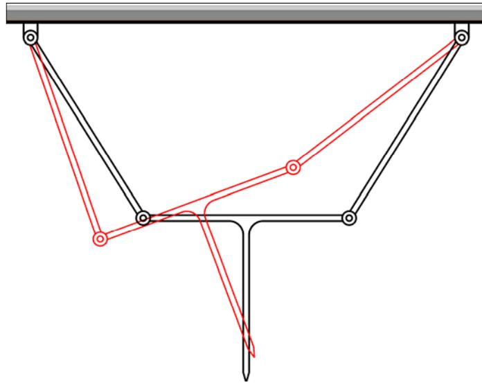
**Figure 6.** Two-dimensional simplified version of nozzle tip pivot, showing two positions
