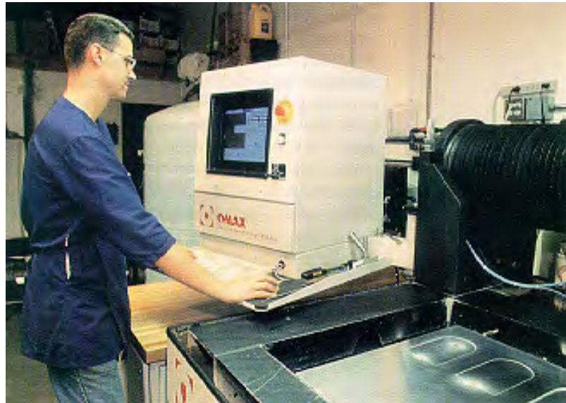
Operator checks CNC screen for program details on OMAX JetMachining operation for machine parts
