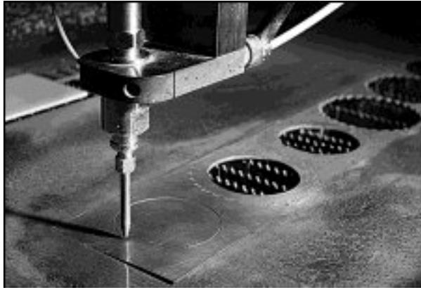
The JetMachining® Center is able to cut a variety of materials, with no toxic fumes or heat-affected zones.
