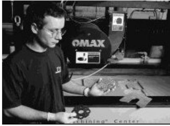
JetMachining® cuts complex geometry part with no secondary processing needed.
