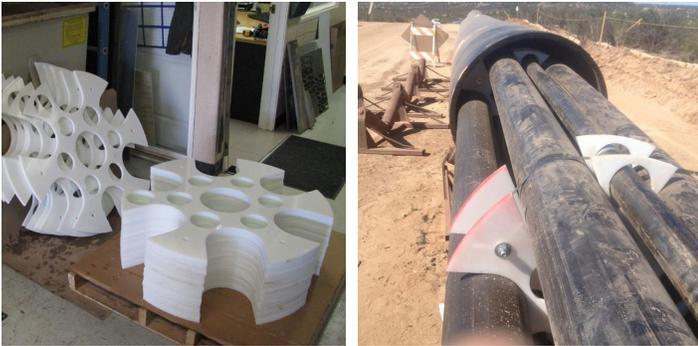
Another market ripe for abrasive waterjet cutting is with hydraulic, pneumatic, and electrical actuators. Factories, plants, and utility companies all utilize these actuators, and often times these are custom built. This means they require custom parts when they break down, and the abrasive waterjet is the perfect solution, with its ability to quickly machine parts in almost any material up to several inches thick.
