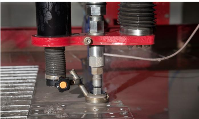
With abrasive waterjet technology, Hough now handles a wider range of production runs, including fast prototype development. He is able to quickly turnaround highly accurate parts without the hassle of tool changes or complex fixturing. Plus, as compared with his other production equipment, abrasive waterjet cutting generates much smoother surface finishes, which eliminates the need for secondary machining in many instances.
