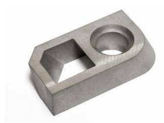
The A-Jet makes cutting bevels simple, and software controls help to eliminate taper.
